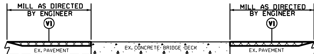
DETAIL 2 BRIDGE MILLING
